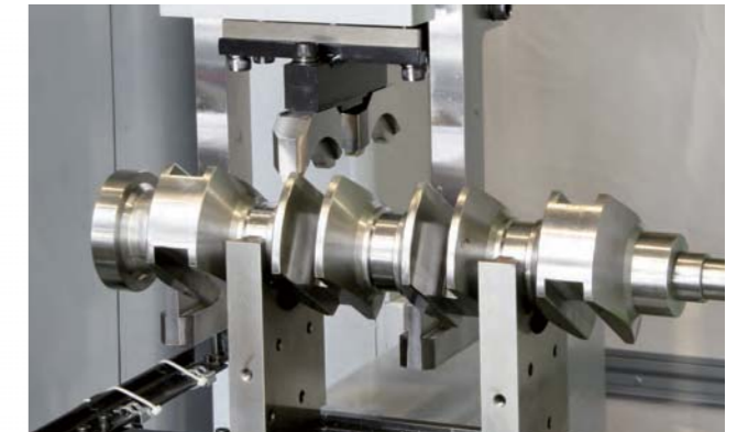
Hand type exclusive for crankshaft workpiece
