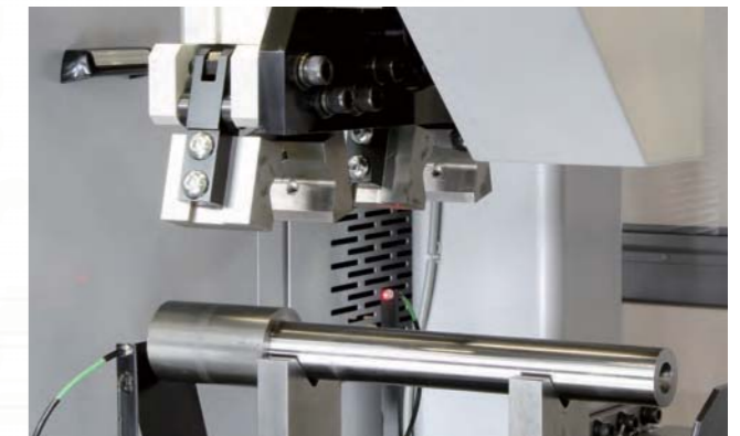
Hand used for shaft workpiece (Pendulum Type)
