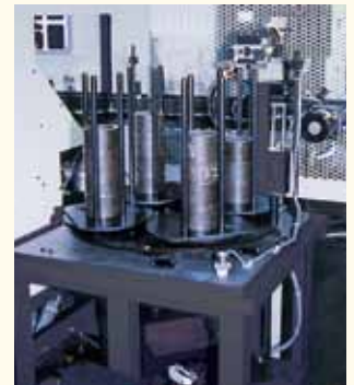
● Rotary Stocker The space-saving, low-cost stocker. The position can be adjusted easily according to the size of the part.
