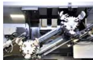
Intermediate turnover unit that can handle large-diameter workpieces
